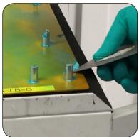
Loosen (if necessary with a spatula, scraper or similar) the sealing film at the edge of the carrier or chamber element that you can grasp the film with two fingers.
