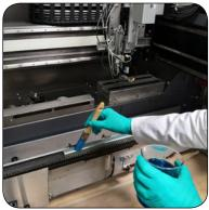
If you want to seal sheets / covers in the chamber of a coating system, proceed as described above: distribute CarrierSeal® evenly and comprehensively on the aereas / machine parts that you want to seal.
