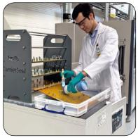
Dripped off CarrierSeal® residues can be easily removed after drying from the CS Workmate parts as previously described.
